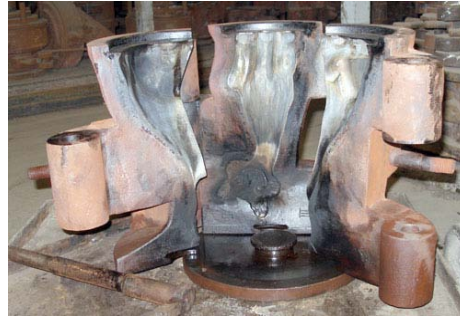
The cast iron Alley Cat mould weighs approximately 250 pounds.
