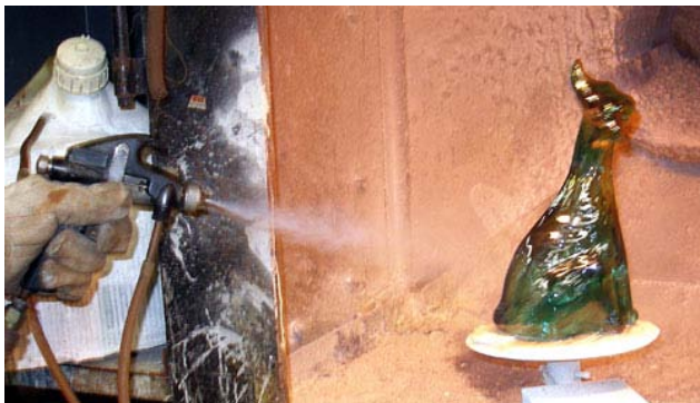
Iridizing: The spray of metallic salts gives our Alley Cat extra sparkle!
