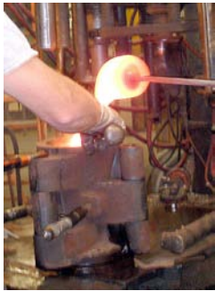
The Gatherer gathers enough glass to flow into the mould, and the presser cuts off the proper amount.
