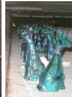
Reheating is done before the iridizing process.
