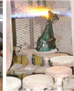
Reheating is done before the iridizing process.
