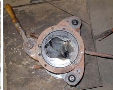
The cast iron Alley Cat mould weighs approximately 250 pounds.
